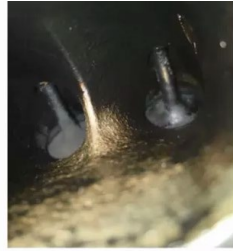
进气门积碳 Intake valves carbon deposition.
